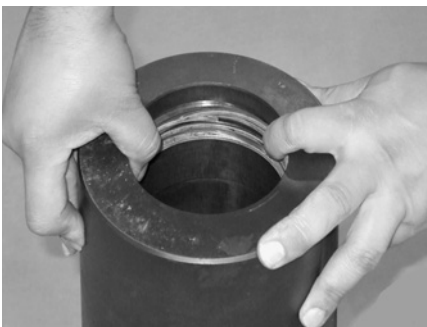
Spread the ring from the center out towards the ends. Press the ring into the groove with the thumbs until the ends meet and the ring is firmly seated in the groove.
