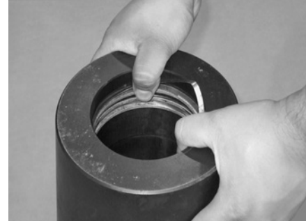
Insert one edge of the seal protector ring into the groove. Insert the opposite edge and press down until entire ring is in place.
