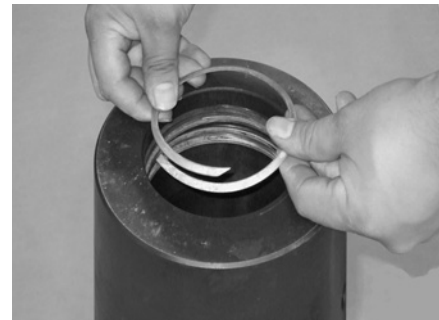
Overlap the ends of the ring until the diameter fits inside the body. Place the edge of the ring opposite the split into the lower groove. Be sure the beveled side of the ring matches the beveled side of the groove.
