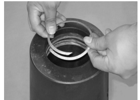
Overlap the ends of the ring until the diameter fits inside the body. Place the edge of the ring opposite the split into the lower groove. Be sure the beveled side of the ring matches the beveled side of the groove.
