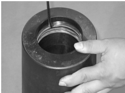
Straighten and flatten the seal protector ring by pressing against it with the bent-tip installation tool (Logan Part No. J1073) from the Jar Service Kit.
