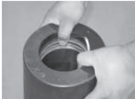
Insert one edge of the seal protector ring into the groove. Insert the opposite edge and press down until entire ring is in place.
