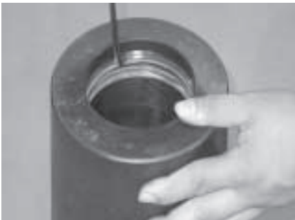
Straighten and flatten the seal protector ring by pressing against it with the bent-tip installation tool (Logan Part No. J1073) from the Service Kit.
