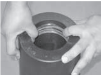
Spread the ring from the center out towards the ends. Press the ring into the groove with the thumbs until the ends meet and the ring is firmly seated in the groove.
