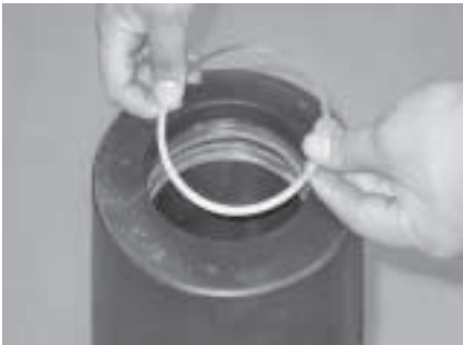
Repeat the installation sequence for the seal protector ring.
