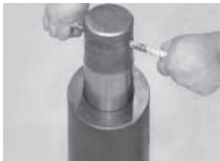
Insert a bar or rod through the top of the setting tool to make handles to hold the tool.
