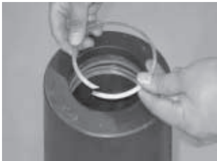
Grasp the non-extrusion ring between the thumbs and forefingers.
