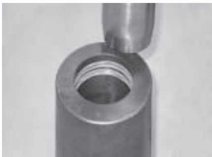
Place the setting tool in a sling and position it over the top of the mandrel body/washpipe body.
