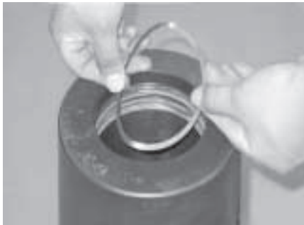
Bend the seal protector ring until it is small enough to fit into the bore.
